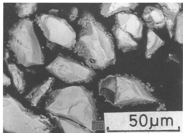
Fig. 1 Morphology of tungsten carbide clad with cobalt powder
